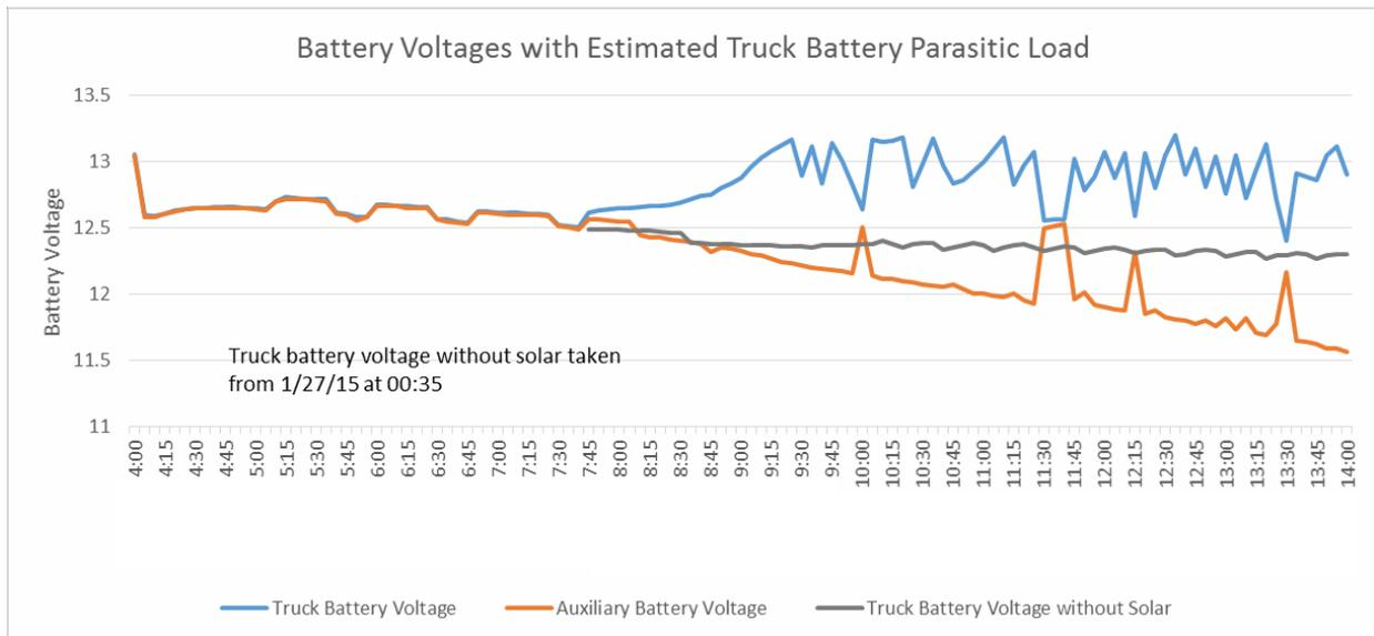
Figure 6: Battery Voltages with and without Solar
