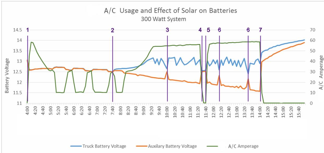
Figure 4: Battery Voltages and A/C Current
