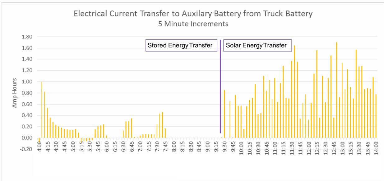
Figure 5: Energy Transfer to Auxiliary Battery
