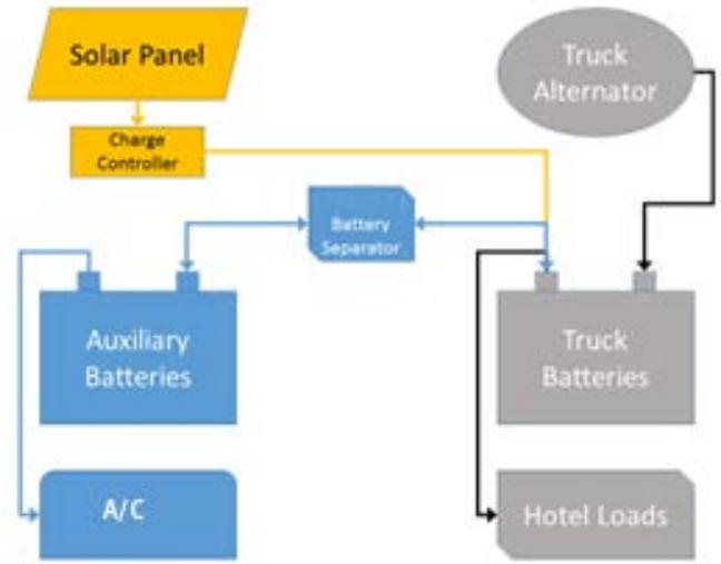
Figure 2b: Solar Connection to Truck Batteries
