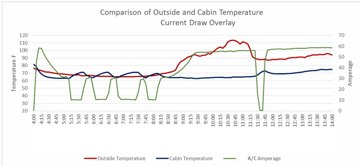
Figure 3: Temperatures and A/C Current Draw
