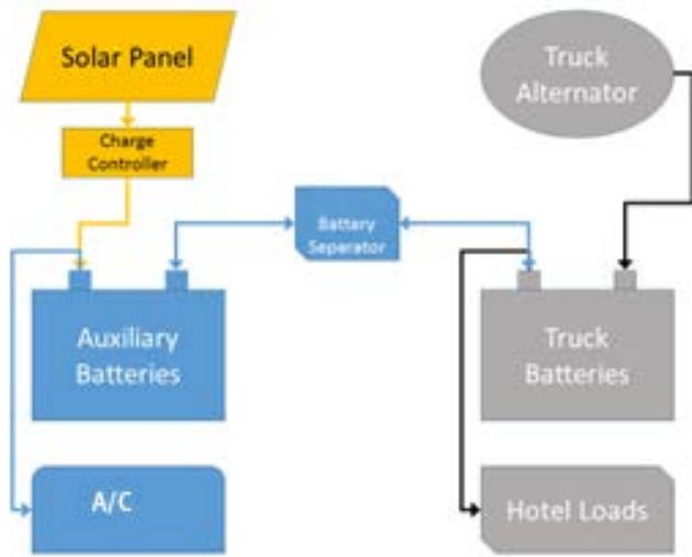
Figure 2a: Solar Connection to Auxiliary Batteries
